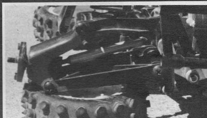
Left: the underside of the chassis. The overall length of the 'Hot-shot' is 15in. The width 9\frac{1}{4} in. Above: close-up of the drive shaft which passes through the R/C crate to transmit drive to the rear wheels. The drive shaft is fitted with hexagon heads similar to those used on the 'Frog.'
