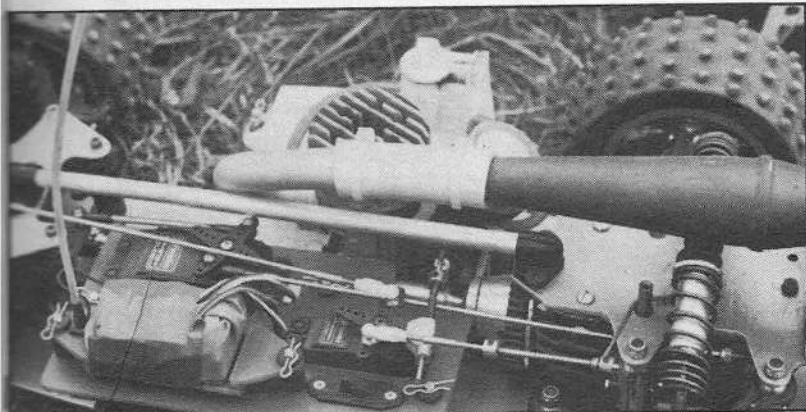
Above left: close up of Stephen Marr's double steering servo set-up on his Serpent 'Cobra.' Left: the revised radio plate devised by Geoff Lindstrom for his 'Mustang Xi2' to allow for a more linear throttle movement between servo and carburettor.
