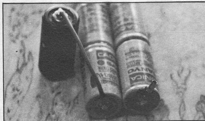
Top: the simplest method of wiring in a seventh cell for modified class racing. First open up an existing six-cell pack. Above: connect the extra cell to one of the terminals. Make sure you connect positive to negative or vice versa. Below: place cell on top with connection at the rear. Bottom: cover the whole pack with shrink wrap. For extra rigidity run a bead of superglue along the touching edges of the extra cell.
